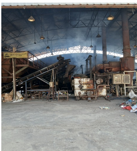
Figure 7. Pyrolysis machine at banyumas TPA producing dense smoke. Source Irwan Hidayana, August 2024.
